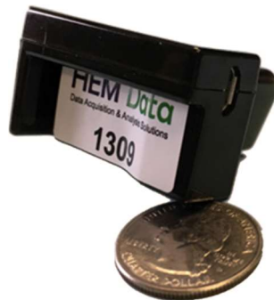
Figure E20. HEMData Data Logger
