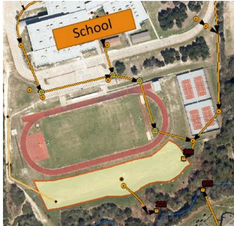
School activities discharge to detention pond and then into Bee Branch
