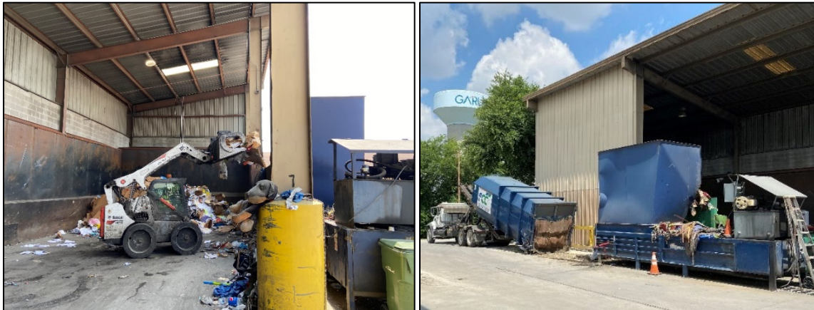
Figure 5-3: Skid Steer Loader Operation and FCC Servicing Compactor Unit
