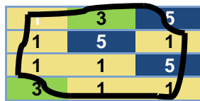
Figure E.1: Subwatershed scores were calculated by averaging the grid cell scores to create one value for each VEIL layer. The bold line represents a watershed boundary.
