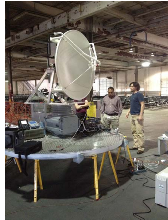
Low power, multi-Doppler, Dual Pol, X-band radars
