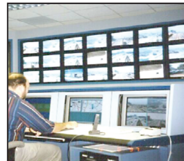
Transportation Management Centers help monitor the performance of the transportation system, quickly responding to incidents.
