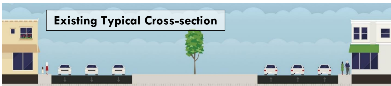
Existing typical cross-section with unprotected and sporadic sidewalks, 12-foot travel lanes, and wide median.
