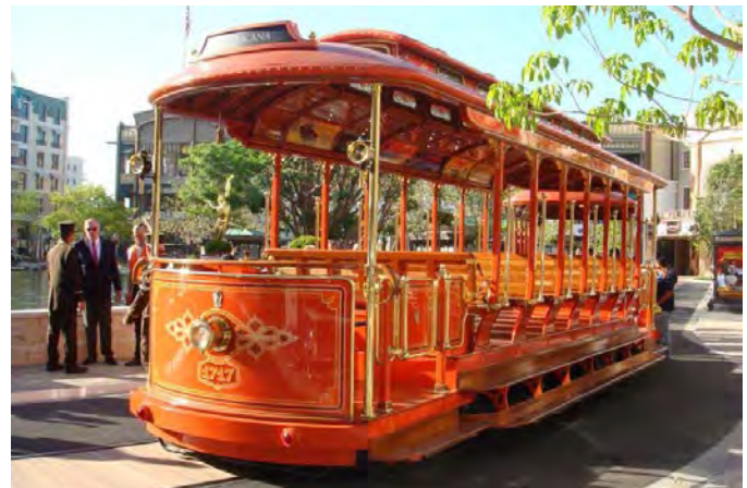
An example of a replica streetcar that is battery-powered. Image source: www.triplannermag.com
