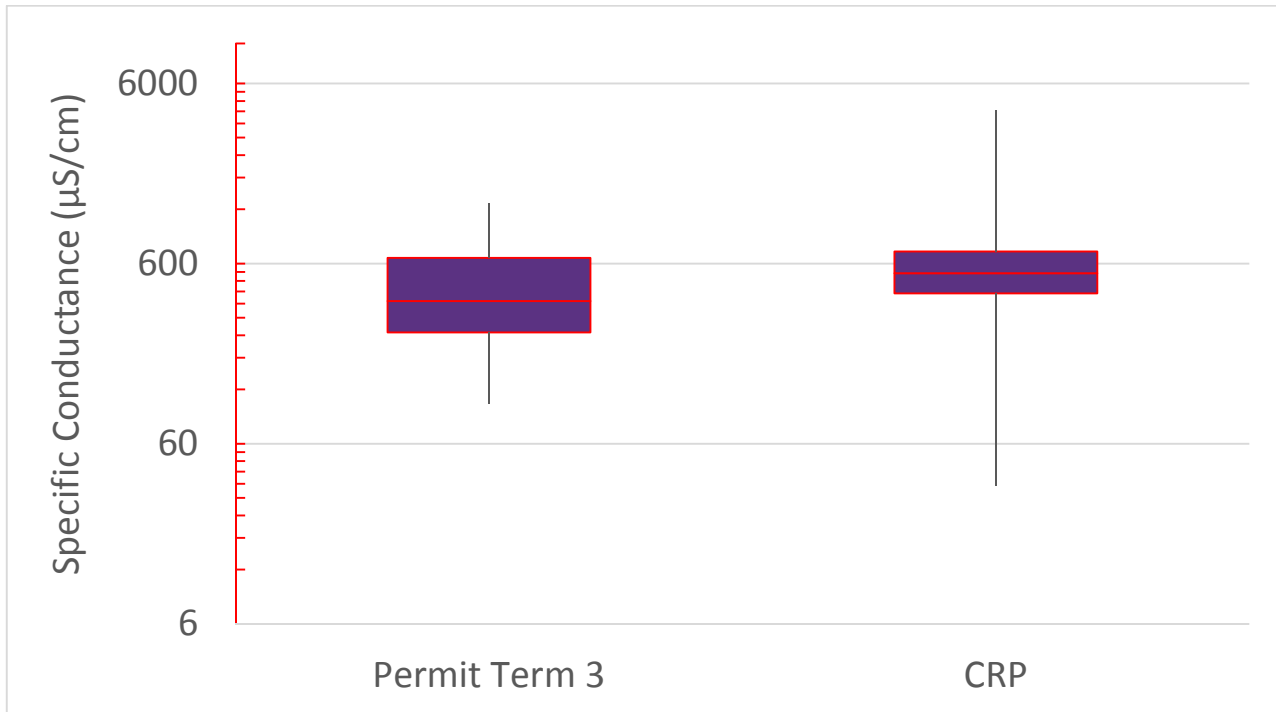
Figure 4-18 Boxplot Comparing Wet Weather Chemical Monitoring Third Permit Term and CRP Specific Conductivity Data at Johnson Creek
