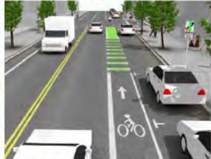
Green Bike Lanes Through Conflict Areas
