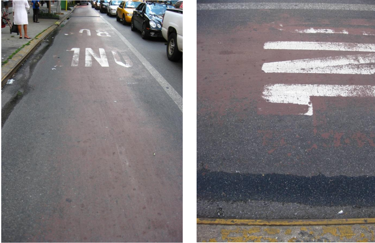
Figure 4. Product ID #1 Wear at a Bus Stop at 34 th Street at Second Avenue
