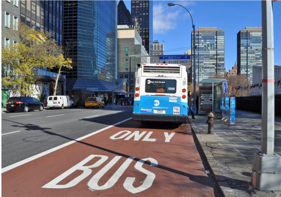
Figure 1. Example of a Red Bus Lane on First Avenue in Midtown Manhattan
