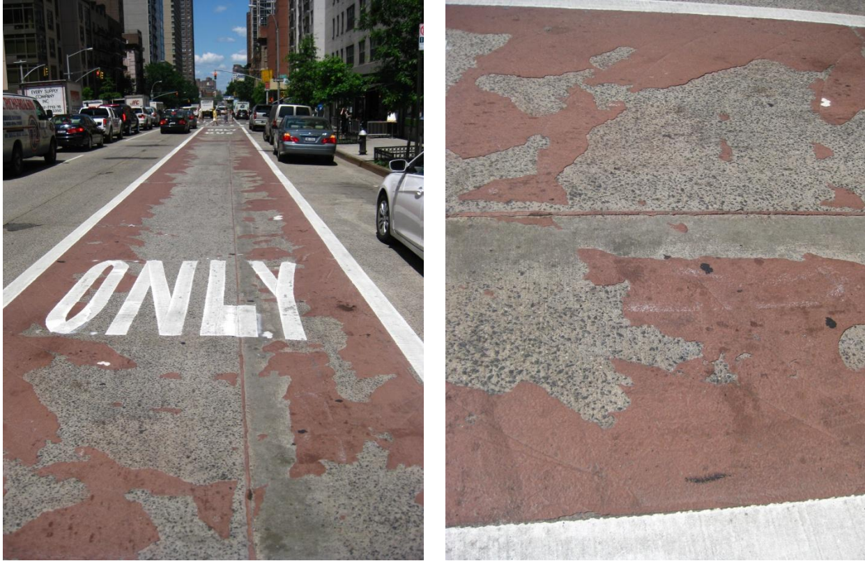
Figure 6. Product ID #6 applied to First Avenue between 88 th and 89 th Streets after Nine Months
