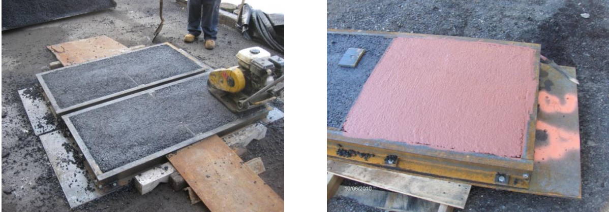
Figure 8. Forms for Red Bus Lane Specimens (left) and Red Bus Lane Product Applied to Asphalt Specimen (right)
