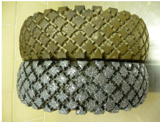
Figure 9. Uncoated Pneumatic Rubber Tire (top) and Silica-Carbide-Coated Tire (bottom)
