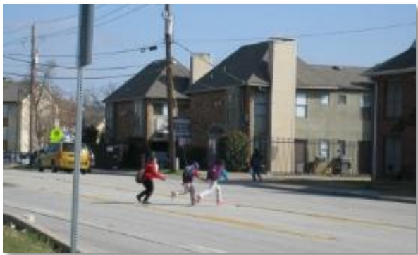
Elementary school students running across 5 lanes of traffic in a midblock location on Park Ln. lacking pedestrian crossings.
