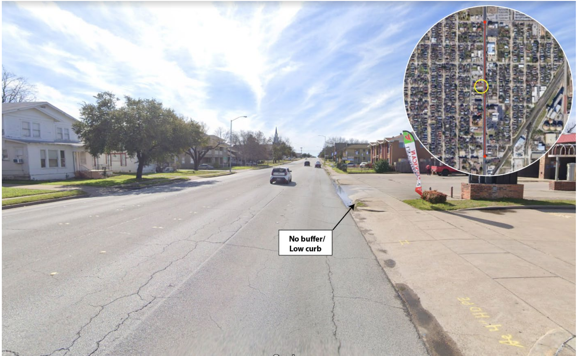
Figure 2: Existing pedestrian facilities lack ADA compliance and lack a buffer between road and sidewalk. Curbs are low and road striping is non-existent.
