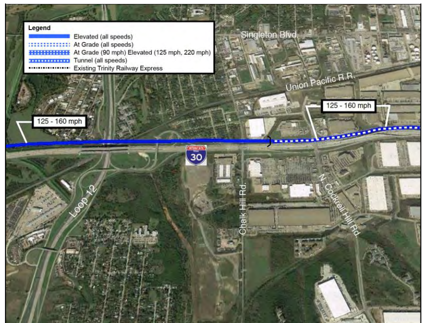
Figure 3-12: Transition to Tunnel at Chalk Hill Rd
