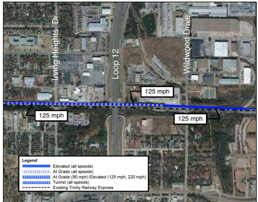
Figure 3-28: Alignment at Loop 12
