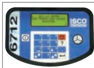
The 6712 Controller is an SDI-12 logger. Manual pump operations are now located on the front panel keys.
