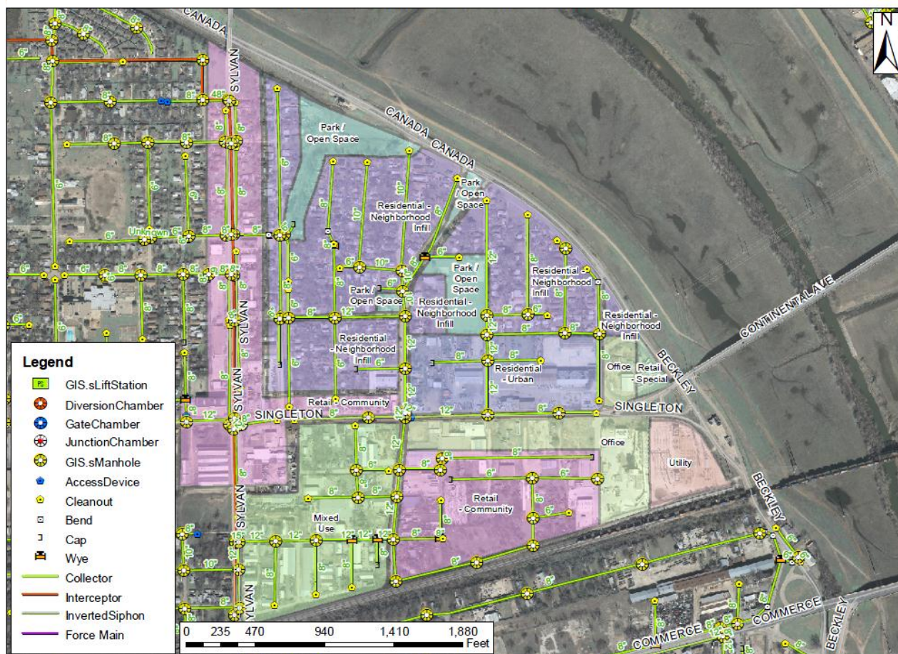
Figure 8: La Bajada/Los Altos Existing Wastewater Infrastructure
