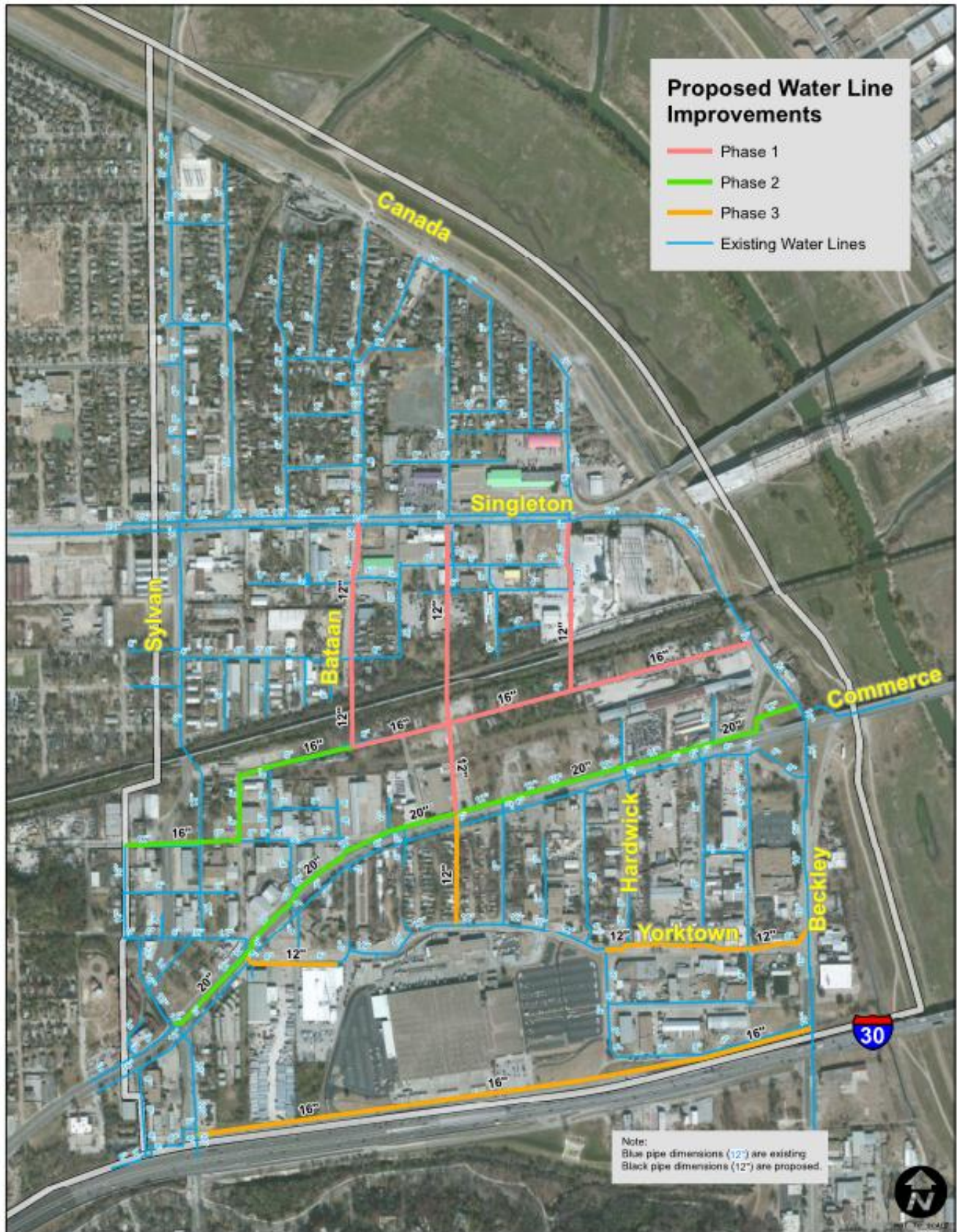
Figure 32: Proposed Water Line Improvements
