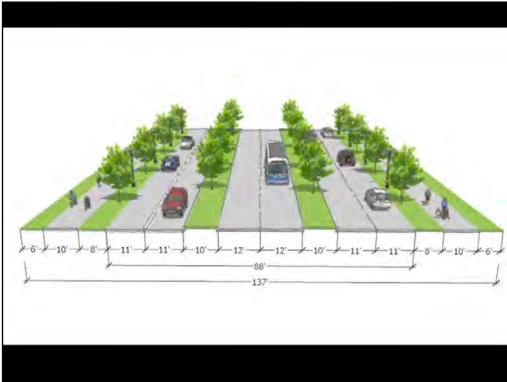
Proposed 199 boulevard section with tree plantings and pedestrian and cycling paths and transit in center.
