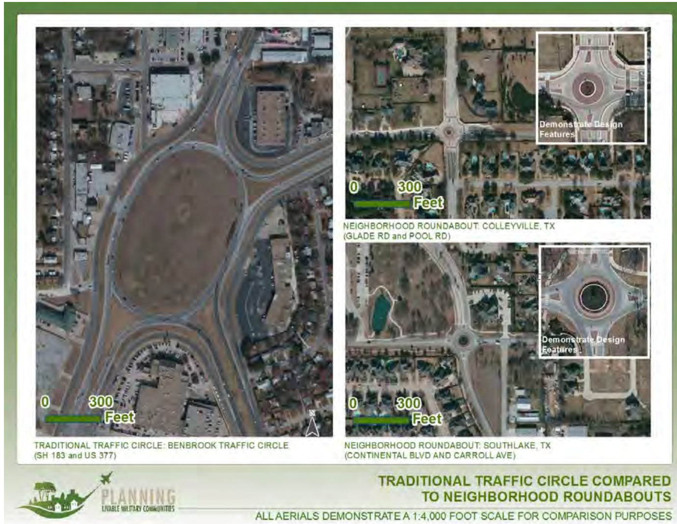
FIGURE 21: TRADITIONAL TRAFFIC CIRCLE COMPARED TO NEIGHBORHOOD ROUNDABOUTS
