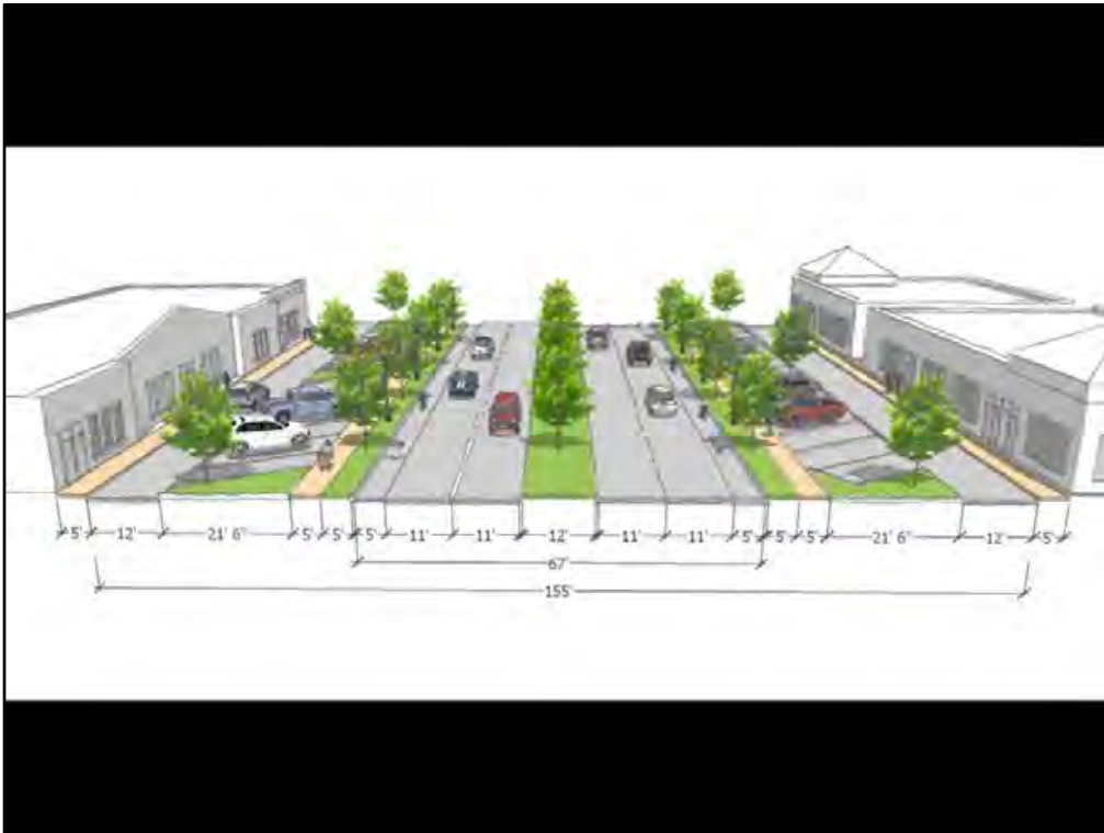
Corridor 183 proposed boulevard street section.
