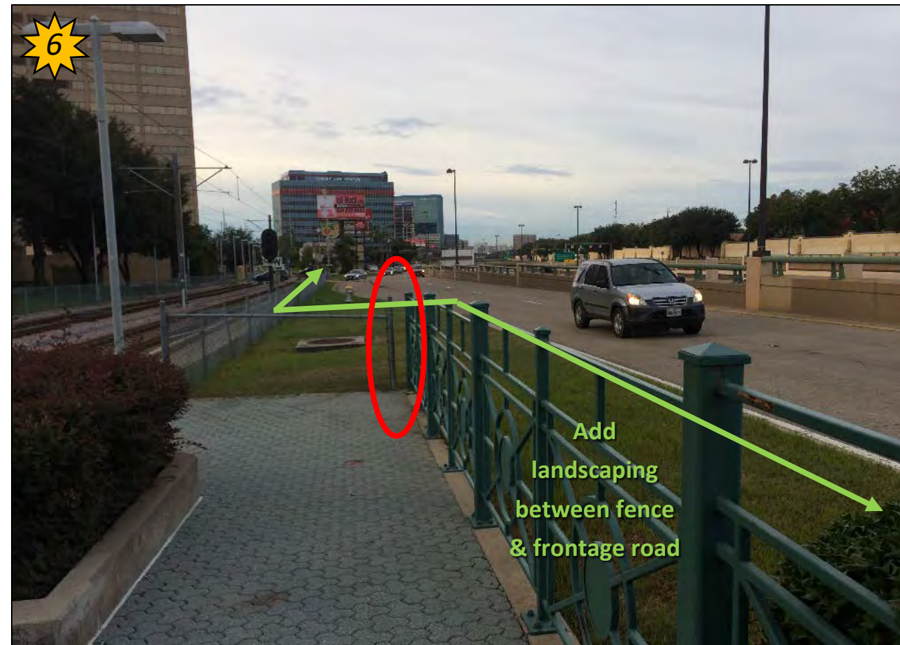
Add landscaping to discourage passenger drop-offs from U.S. 75 frontage road travel lanes. Bent fences indicate existing passenger crossings from Locations 5 and 6.
