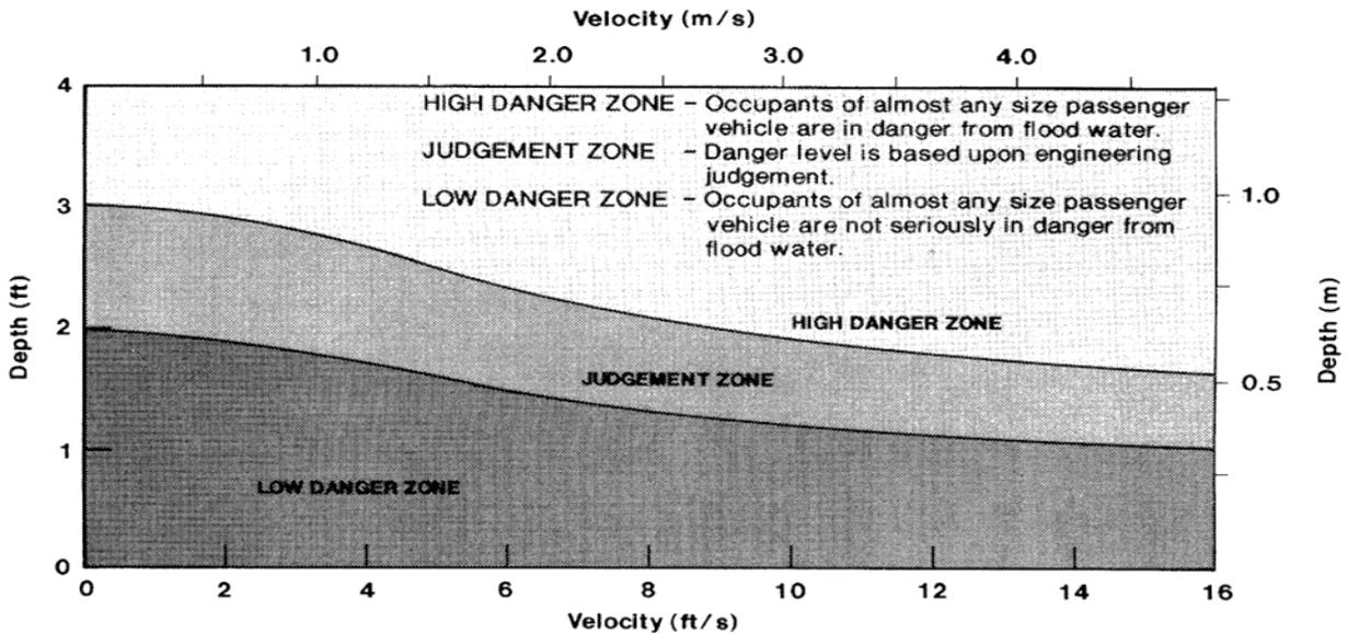
Figure 5-15. Depth-Velocity Flood Danger Relationship for Passenger Vehicles
