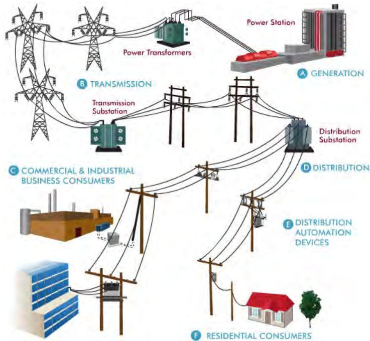
Figure 7-1. Electric Pathway (Source: Oncor)
