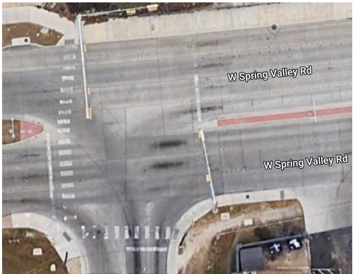
Figure 8: Change in crosswalk direction delineated only with pavement marking at Esperanza Road (Google)
