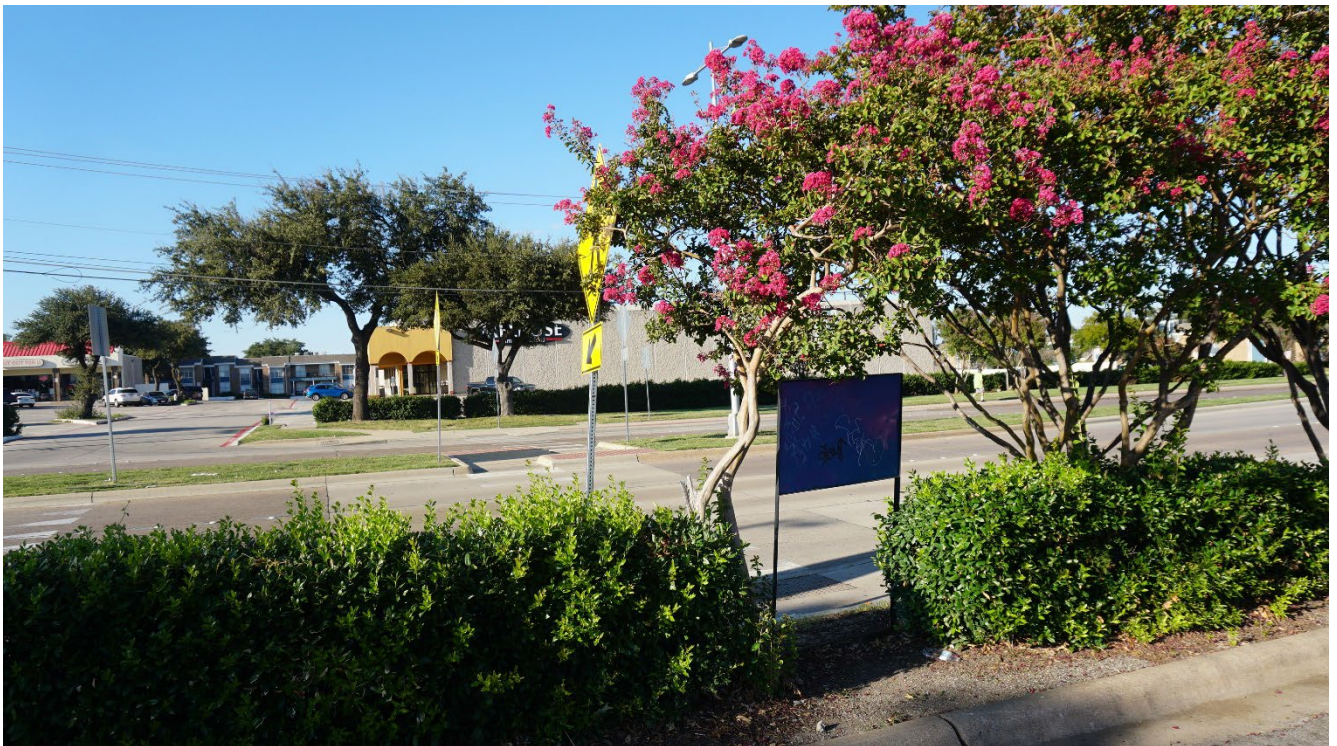
Figure 16: Pedestrian path from western midblock crosswalk/sidewalk into Fiesta is blocked
