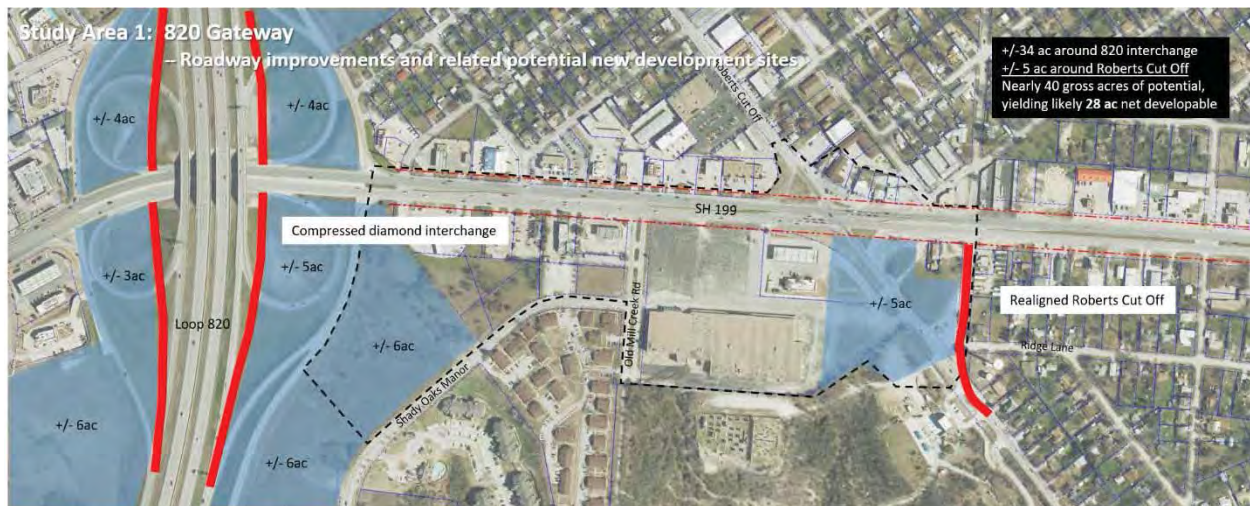
Figure 24. IH 820 Gateway: Roadway Improvements
