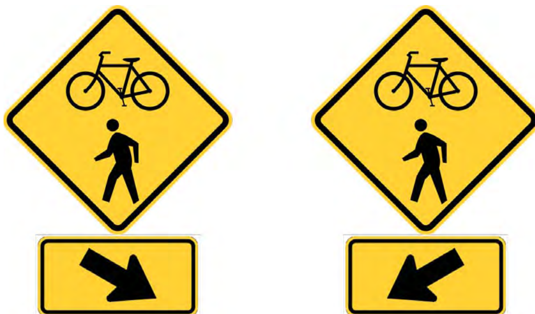
Figure 26. Sign Assemblies with W11-15 and W16-7P Left and W16-7P Right
