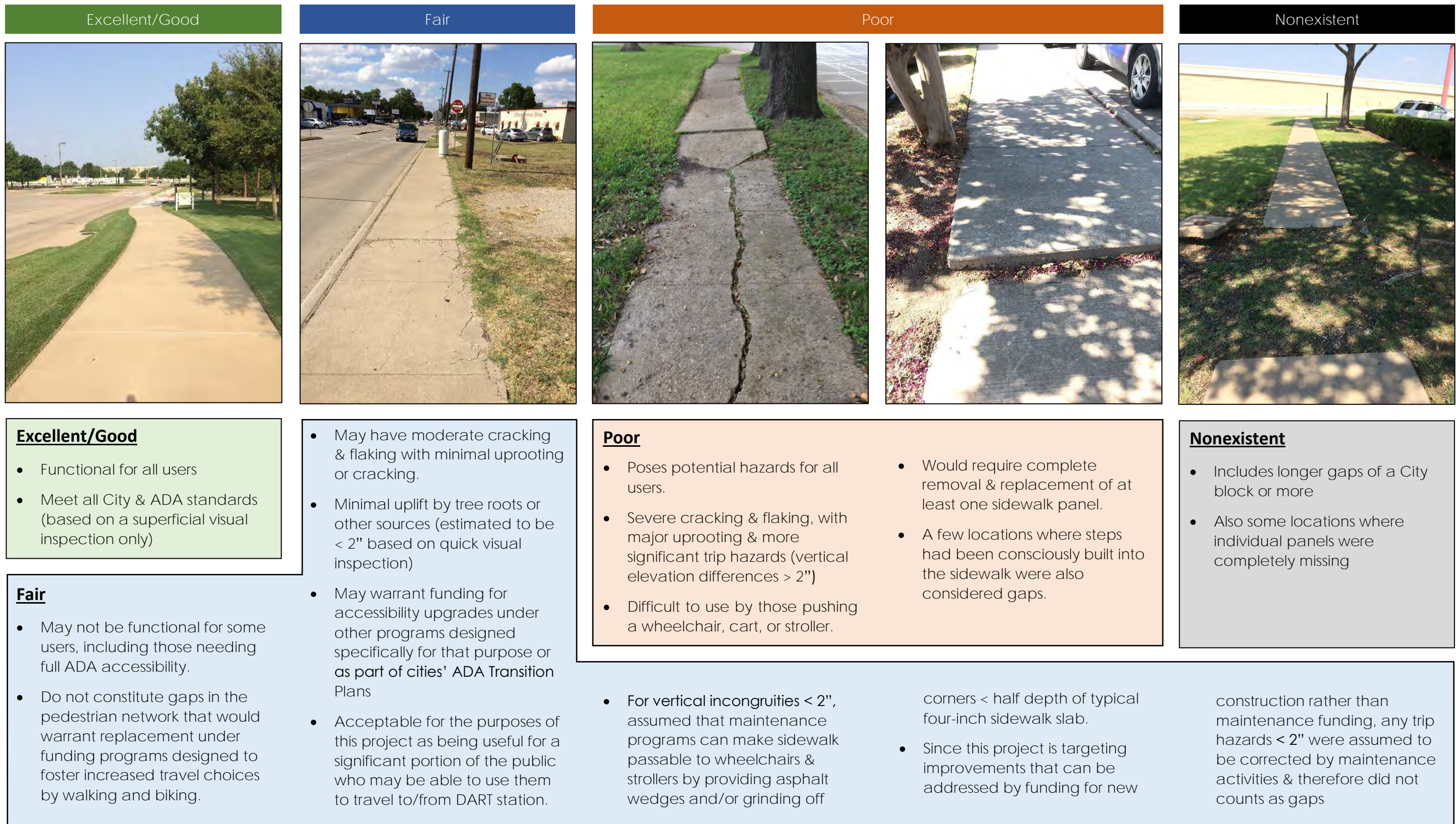
Figure 3: Sidewalk Condition Classification
