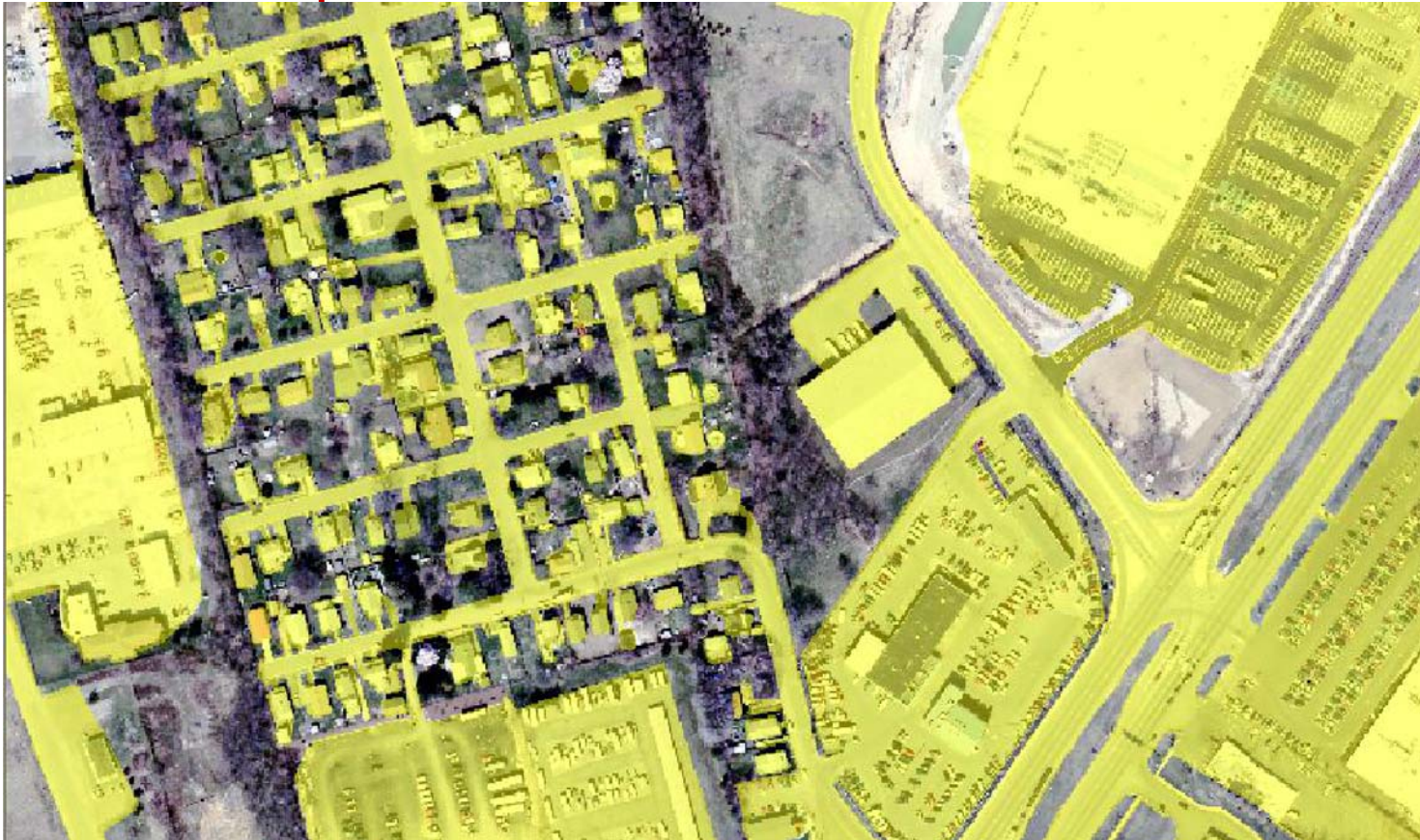
Enhanced automated impervious (1 m pixel size) over ortho imagery for State of Delaware
