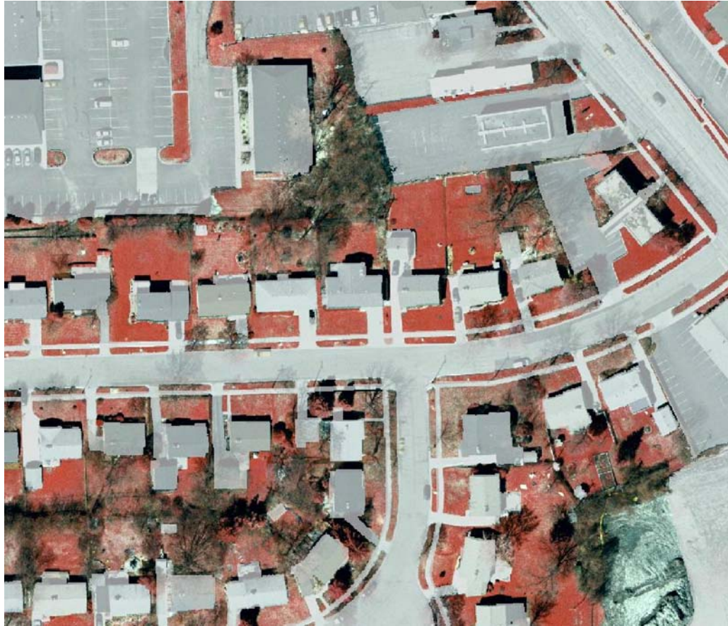
Premium impervious (6" pixels) over 6" pixel resolution ortho imagery for Ann Arbor, Michigan
