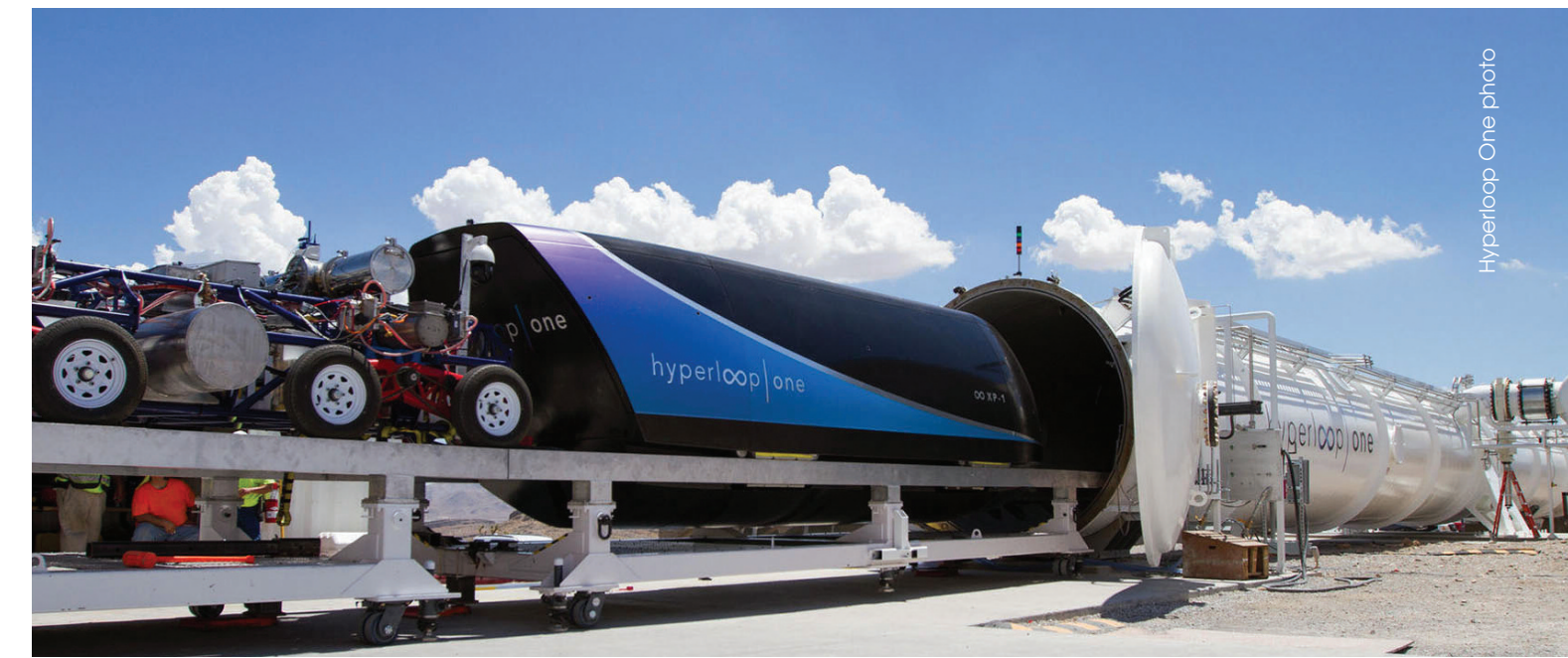
The Regional Transportation Council agreed to consider hyperloop technology as a potential way to link North Texans with the planned high-speed rail lines to Houston and South Texas. Hyperloop relies on magnetic levitation to move people and goods through a low-pressure tube at high speeds.
