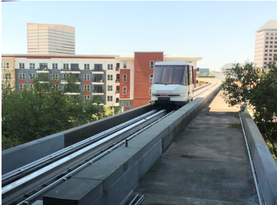
Figure 6.1-1 Las Colinas Vehicle, Guideway, and Proprietary Trackwork
