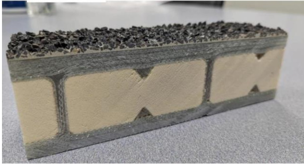
Figure 6.1.2-2 Expanded View of Polymer Deck Panel
