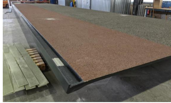
Figure 6.1.2-3 Polymer Panel for Potential Retrofit Deck
