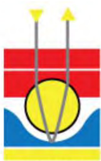
Glass Bead Retroreflection
