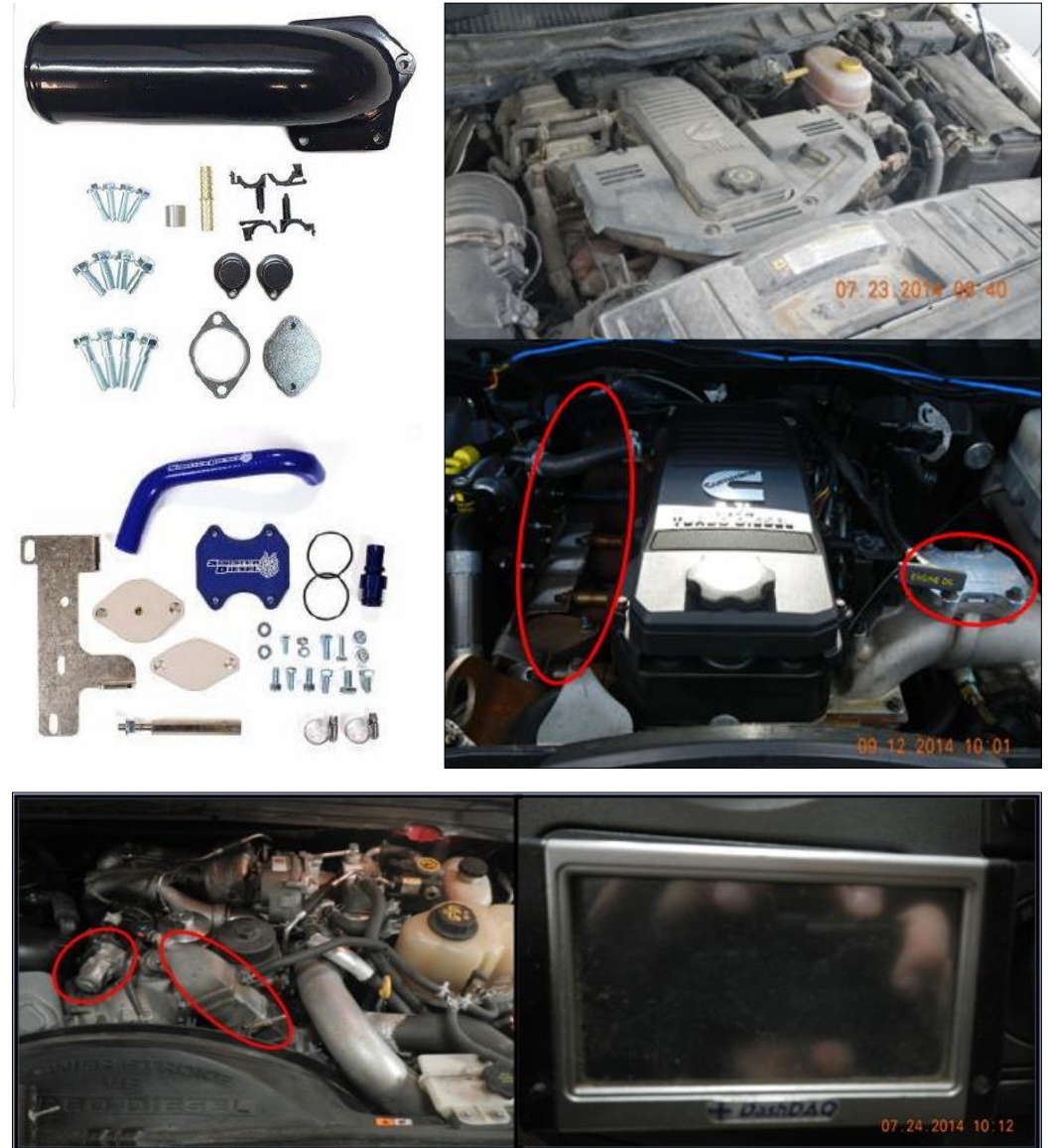
EGR electronic disablement (all EGR parts present and sensors plugged in)
