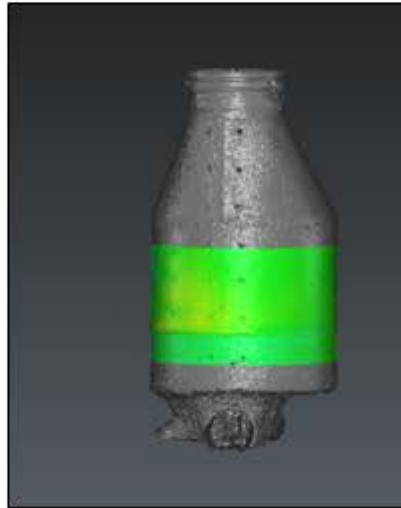
Manhole Virtual Model (MVM™) (Diameter, Elevations, Material)
