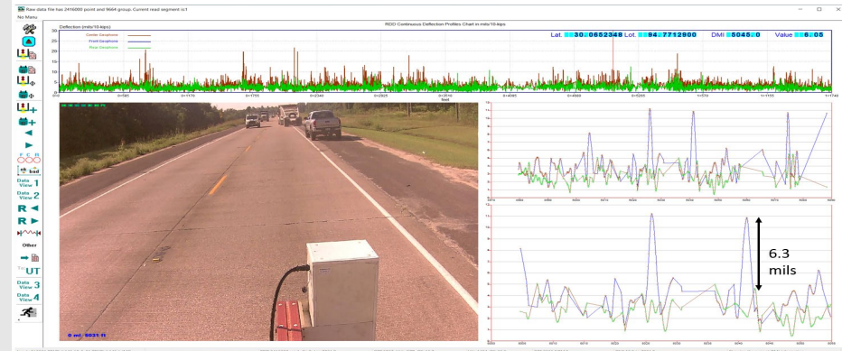
Joint Movement under TPAD loading
