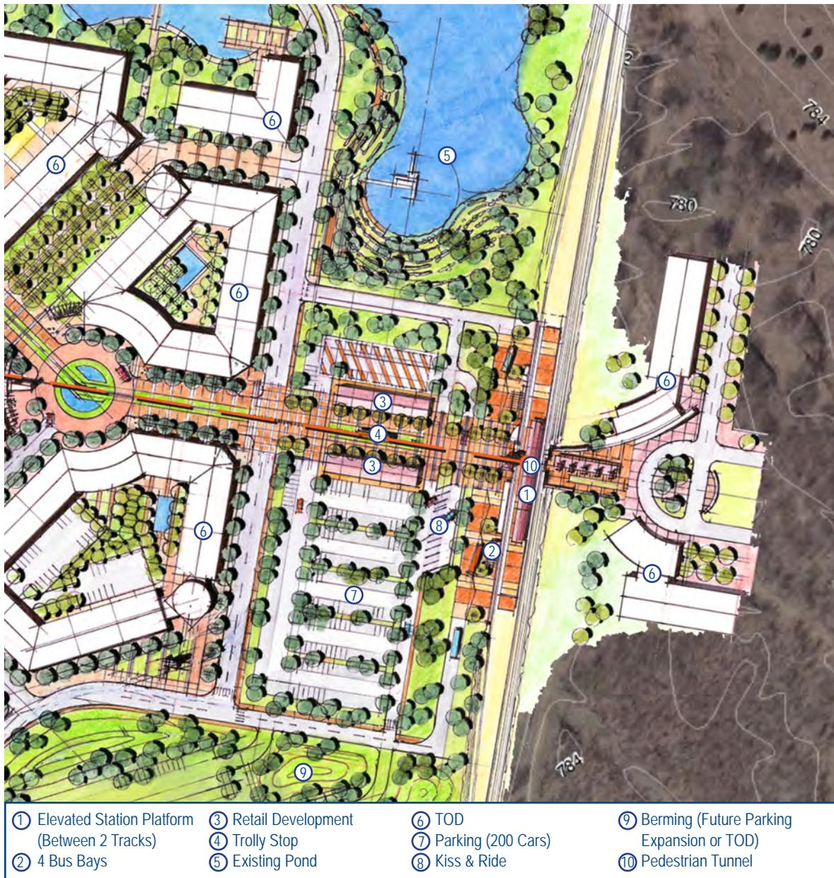
Figure C.5 Detailed Station Site Plan
