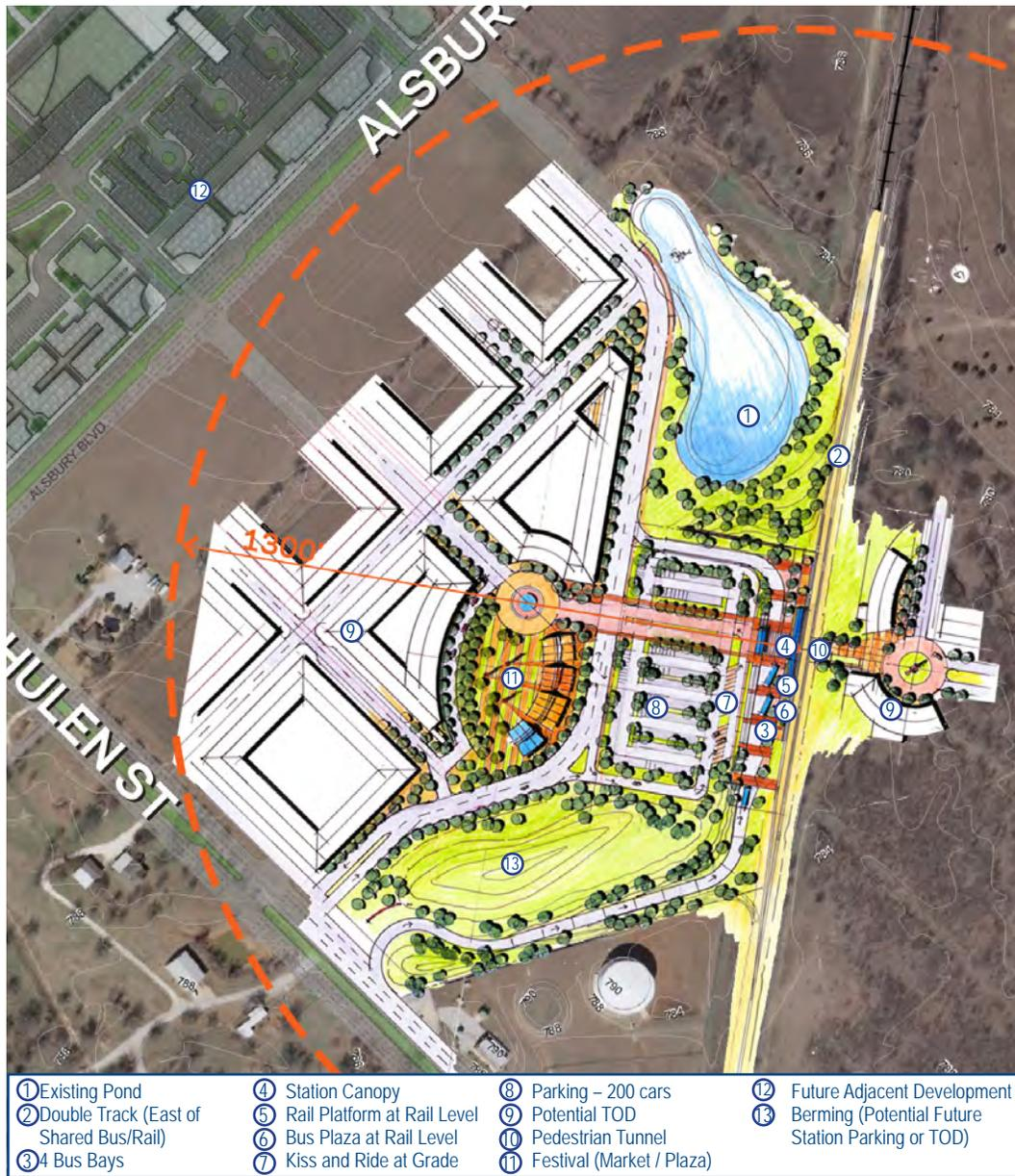
Figure 3.5 Concept B Site Plan
