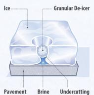
that point, creating a salt/water mix (brine) that continues melting the ice, undercutting the bond between the ice and the road.
