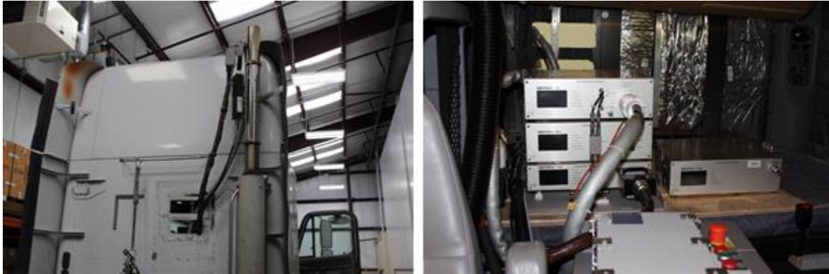
Figure 9: PEMS Installation on Test Truck
