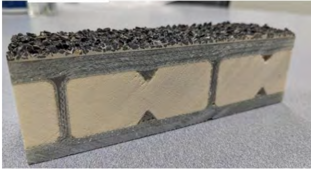
Figure 6.1.2-2 Expanded View of Polymer Deck Panel
