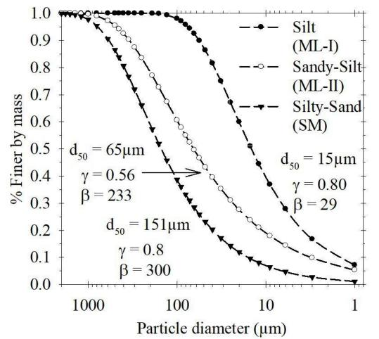
PSDs modeled with gamma distributions using the shape (γ) and scale (β) parameters
