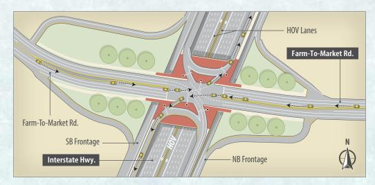
**NOTE:** Each graphic panel represents only the general layout and traffic flow through a SPUI. They are not specific to how the SPUI at US 75/FM 664 will be configured.
