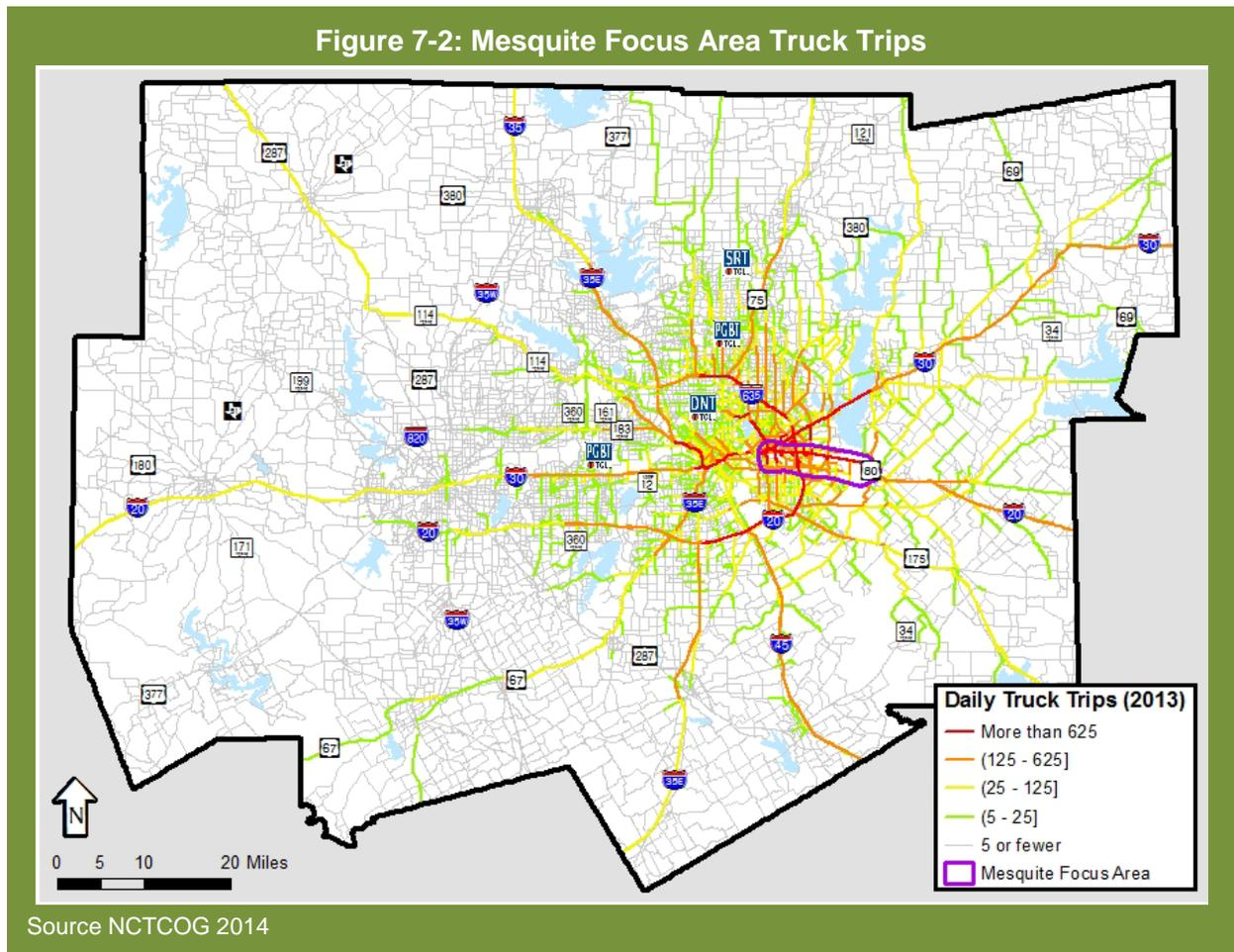
Total daily estimated truck VMTs to and from the Mesquite focus area is approximately 531,807 within the region. Seventy-three percent of the VMTs were estimated to be travelled on limited access facilities. Many of these truck trips continue to out-of-region destinations, increasing total daily truck VMTs from the Mesquite focus area.
