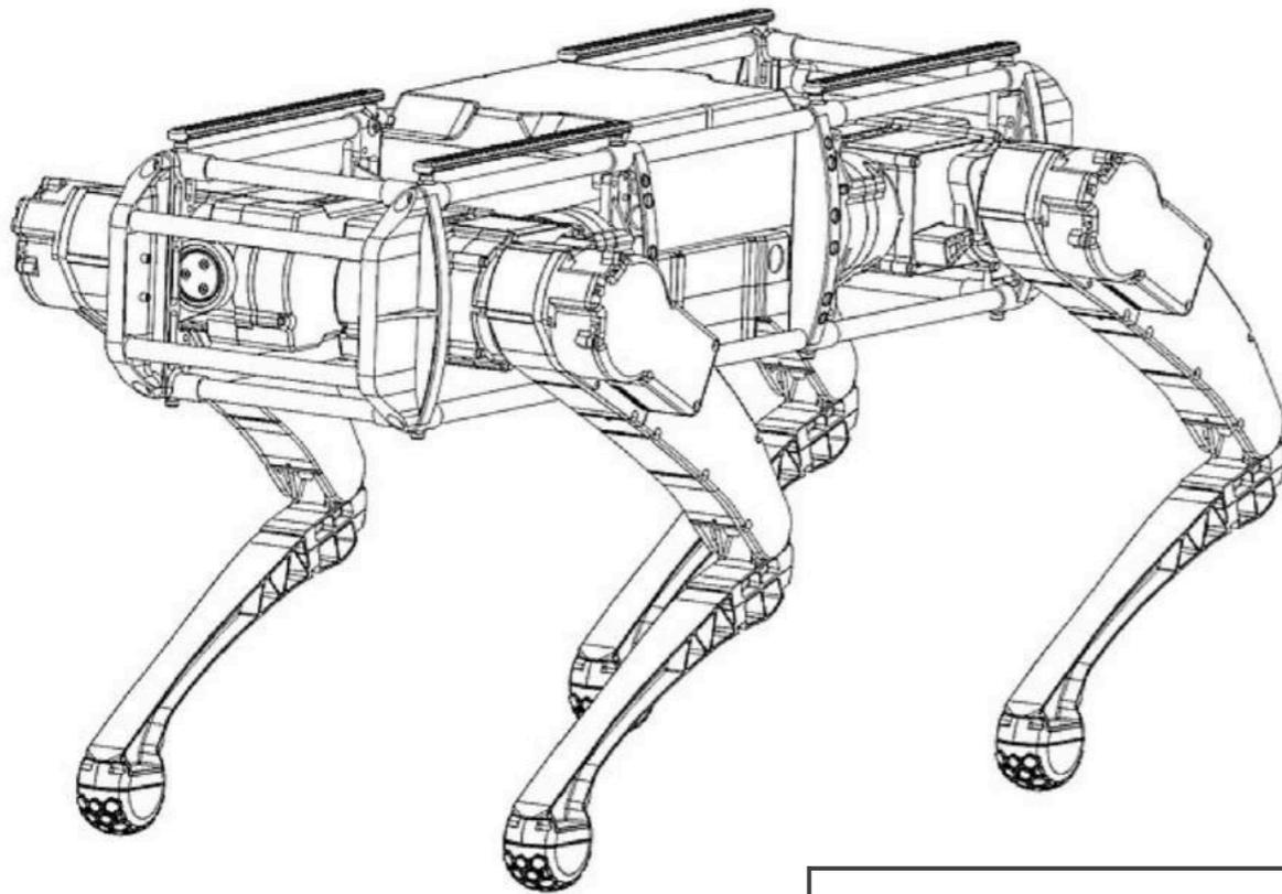
**Long Endurance.** 8 - 10 hrs. mixed use and 21 hrs. standby. Travel 7.5+ miles in 3.5 hrs. on single charge
