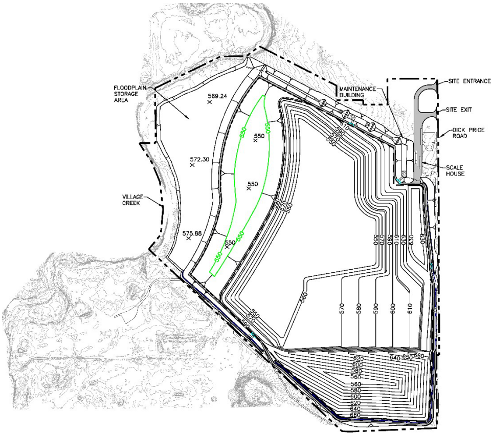
PROPOSED LANDFILL BASE GRADING PLAN
