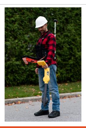
With Eos Locate for Field Maps, utilities can map their buried infrastructure (e.g., electric, gas, water, telecommunications infrastructure and more) with submeter or centimeter accuracy. All a field worker needs is an Eos Arrow GNSS receiver, Field Maps for ArcGIS, and a compatible locator device.
