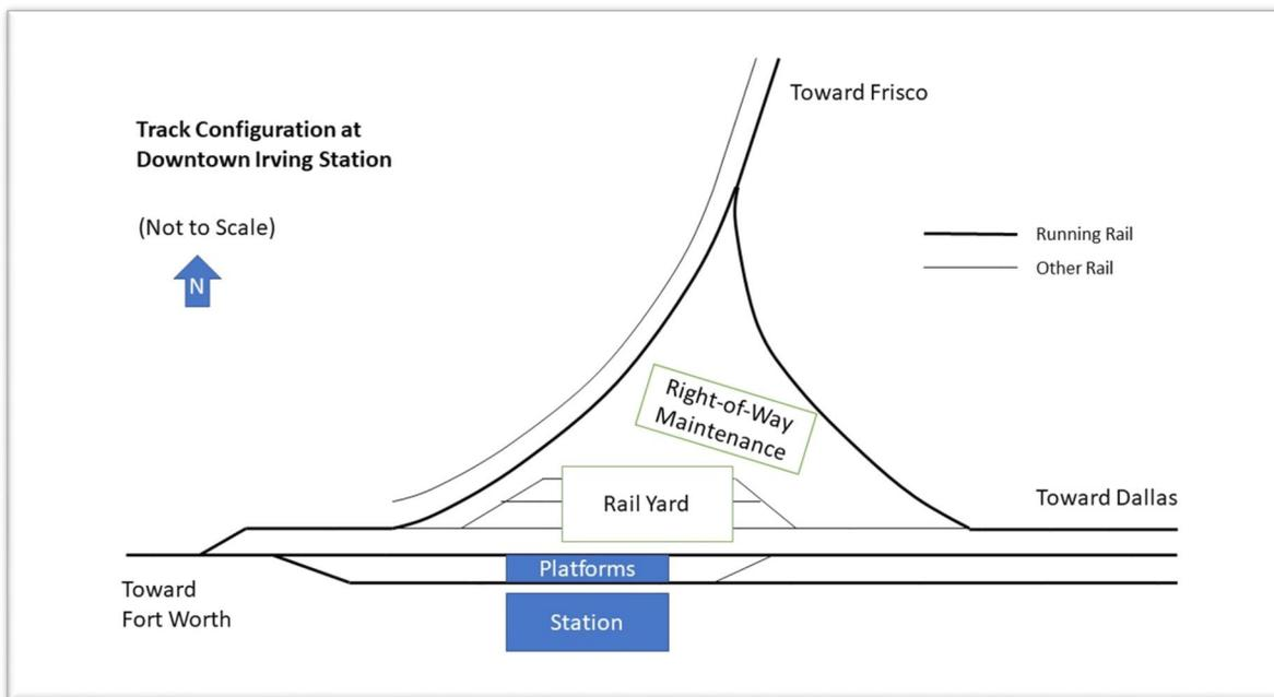
Figure 24: Diagram of approximate track configuration and station location at downtown Irving
