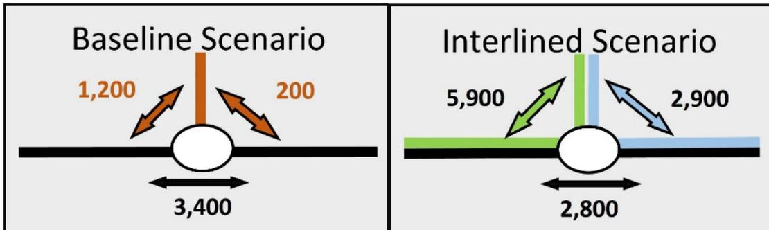
Figure 18: Effects of Interlining at downtown Irving, showing the difference between the baseline scenario (top), in which passengers must change trains if they want to transfer between the TRE line and the Frisco line, and the Interlined scenario, which offers a one-seat ride through downtown Irving regardless of destination.
