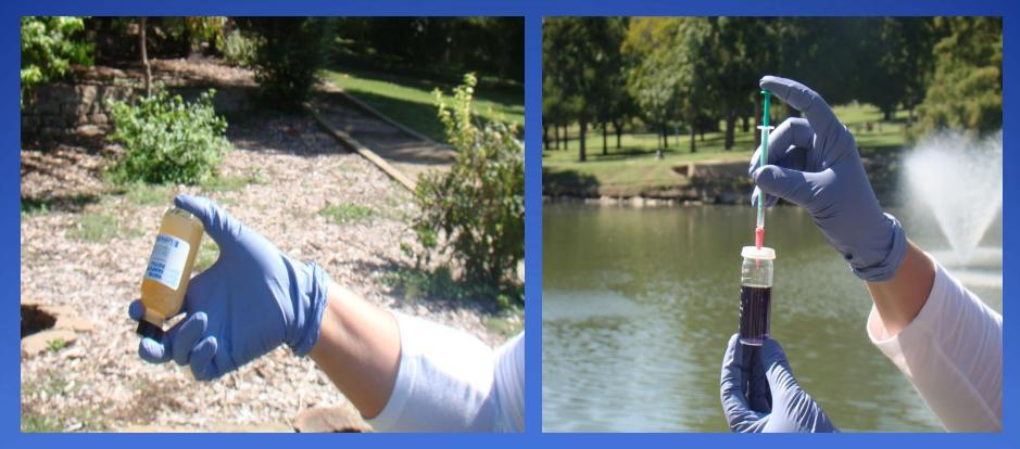
Fill the titrator until the top (not the bottom) of the ring of the green plunger tip lines up with the 0.0 mark (see photo). Check to ensure the plunger does not move
