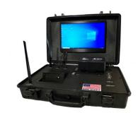
Drone live stream kit. A small, lightweight unit that connects to our incident command system to live stream UAS with 2-way comms and sub half second latency to a HD touch screen on Windows 10 OS. The Credit card sized PC is made in the USA, embedded in a rugged 4 lb case. 1 HDMI input. 1 HD/SDI BNC option available Connections: 4 USB 2.0 - 1 USB 3.0 - 1 RJ45 - 110 A/C - 12V DC adapters - battery option available
