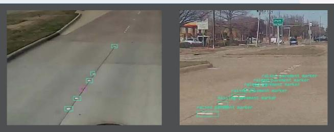
Figure 13. This figure shows show two different examples of missing raised pavement markings
