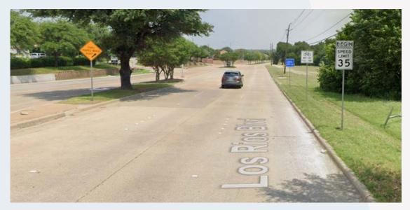
Figure 7. Northbound Los Rios Boulevard at 14th Street- The City of Plano Transportation Division identified insufficient and incorrect use of signs and pavement markings in order for drivers to taper and merge properly for the inside lane drop traveling northbound on Los Rios Boulevard north of 14th Street.
