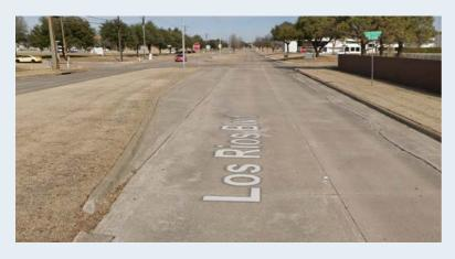
Figure 5. Northbound on Los Rios Boulevard at Merriman Drive– The City of Plano Transportation Division identified missing advanced warning Stop Ahead (W3-1) signs at all four approaches. Per MUTCD Table 2C-4 for a 35 mph condition, the Stop Ahead (W3-1) sign shall be placed 100 feet in advance of the Stop (R1-1) sign.
