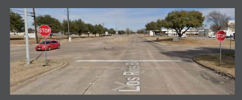
Figure 4. Northbound on Los Rios Boulevard at Merriman Drive– The City of Plano Transportation Division identified that pedestrian ramps were present at all four corners of the intersection, but crosswalk pavement markings were missing at all four approaches.
