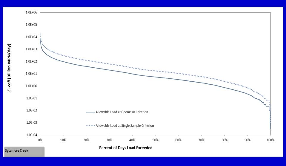
Load duration curve of allowable bacteria, Station 17369
