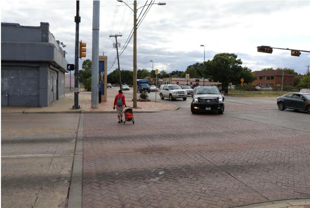
*Figure 7: the sidewalks and crosswalk ramps along MLK don't line up, requiring out of direction travel for some users, along with push buttons in improper locations.*
