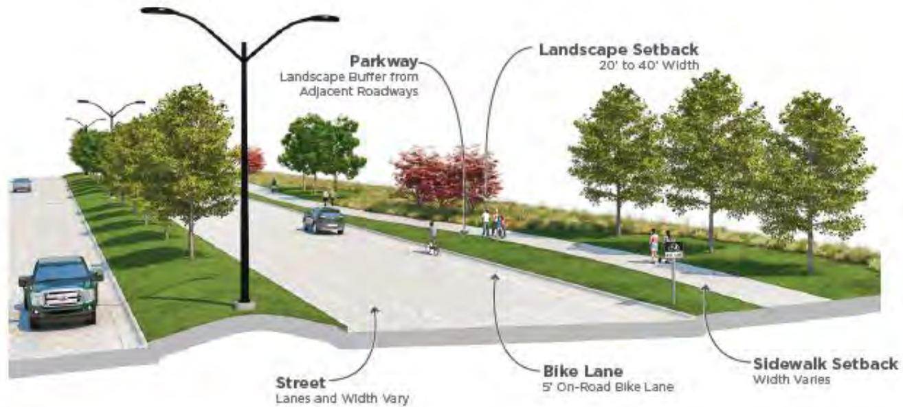
Figure 4.4, Typical Street Edge Condition. (Source: Norris Design)
