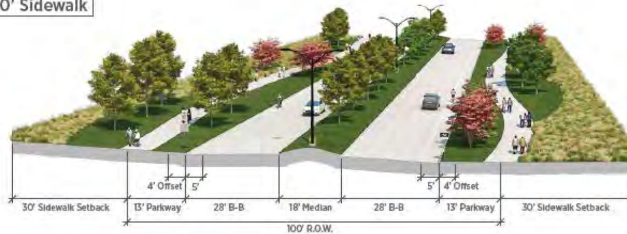
Figure 4.2, Minor Thoroughfare; M4D. (Source: Norris Design)
