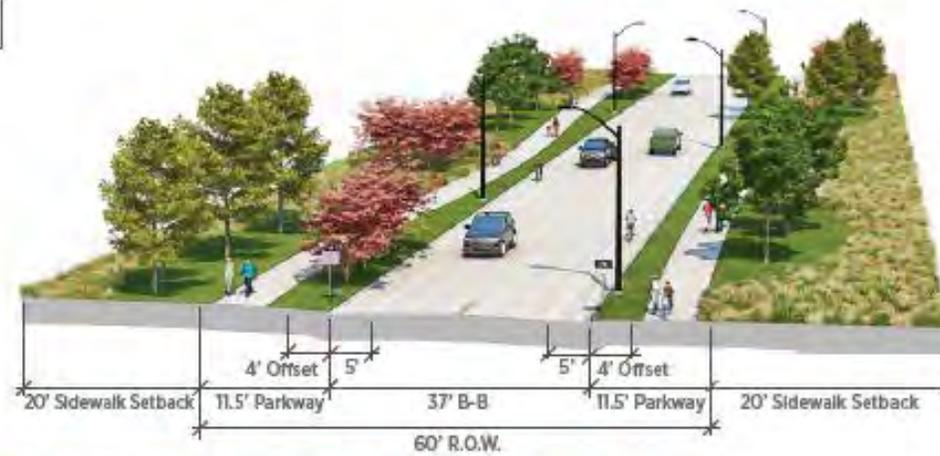
Figure 4.1, Collector Street with Bike Lanes; C2U. (Source: Norris Design)
