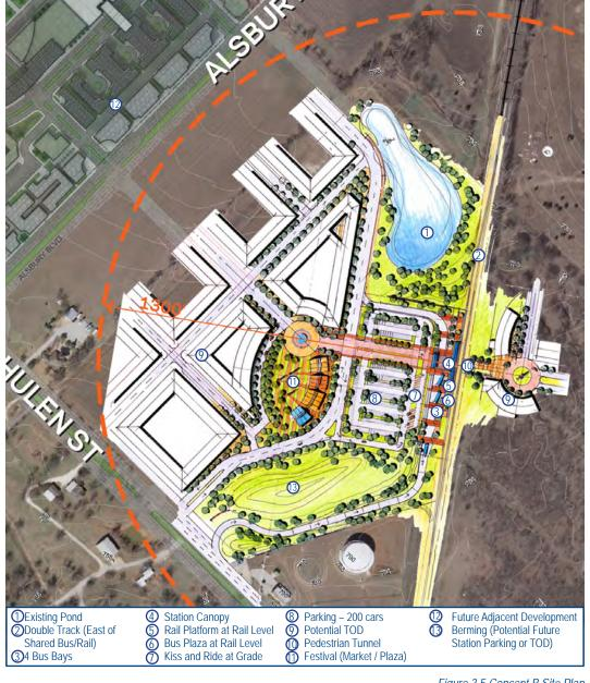
Figure 3.5 Concept B Site Plan
