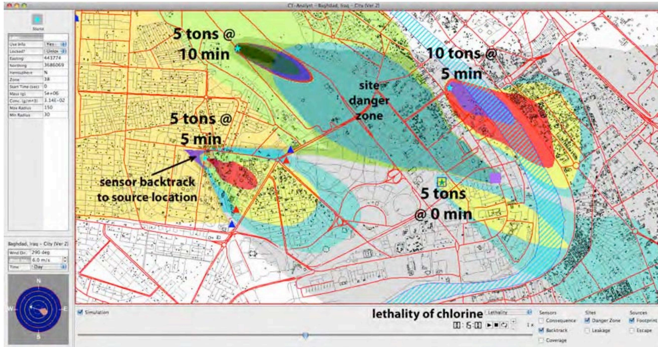
The entire CT-Analyst GUI display predicting lethality for a scenario involving four separate chlorine releases in downtown Baghdad. Notations have been added giving the amounts and release times of the four sources. Sensor fusion for a backtrack computation and a site danger zone are also shown. Computation for this composite display takes about 0.1 second.
