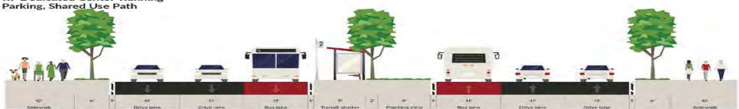
Alternative 2-d Four Lanes w/ Dedicated Center-Running Transit, No Parking, Shared Use Path
