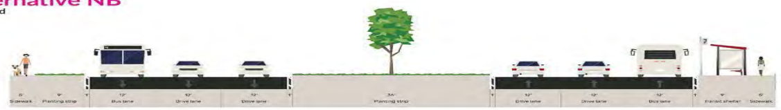
Alternative 2-b Four Lanes w/ Shared Right-Running Transit, No Parking, Shared Use Path
