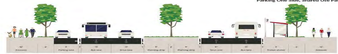
Alternative 2-c Four Lanes w/ Dedicated Right-Running Transit, No Parking, Shared Use Path
