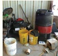
Improper storage of waste fluids.
